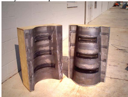
Figure 5. Deposition Screen Utilized to Fabricate F18 Dorsal Cover Preforms (screen shown configured for inner mold line skin).
