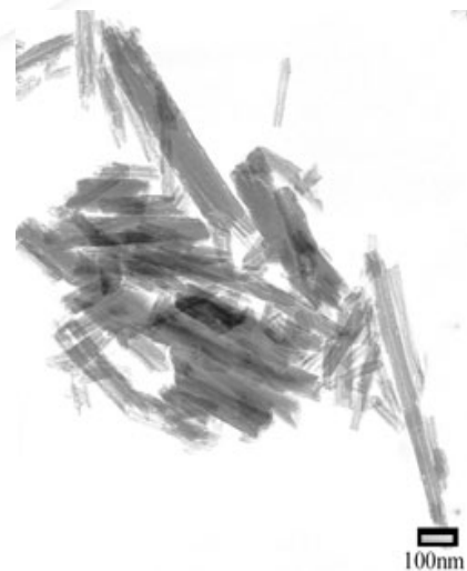
Halloysite nanotubes from Atlas mines in Utah (imaged at Alfred University with transmission electron microscope)
