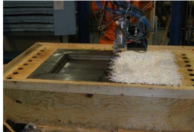
Using NCC’s Rapid Fiber Preforming technology to spray fibers on a preform for a bus side panel.
