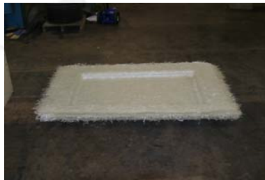
Completed bus panel preform.
